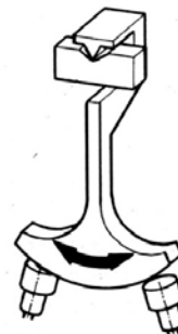
Contact-free and reaction-free measurement of the position or motion of a pendulum.
